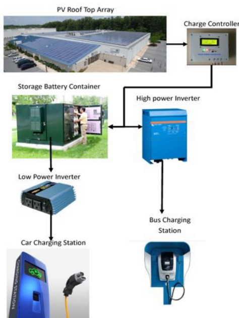
Figure 5: Solar + Storage Microgrid Connected to EVs
